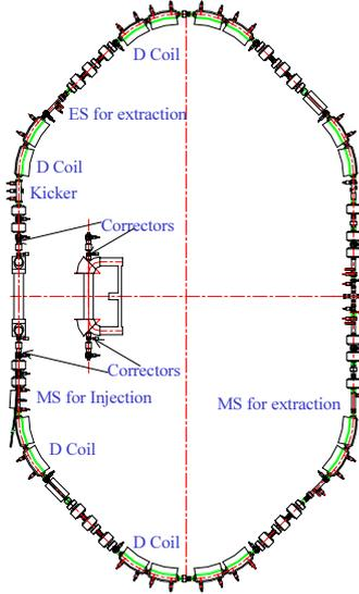
Figure 7: Layout of CSRe injection and extraction
