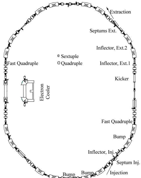
Figure 1: Layout of CSRm injection and extraction
