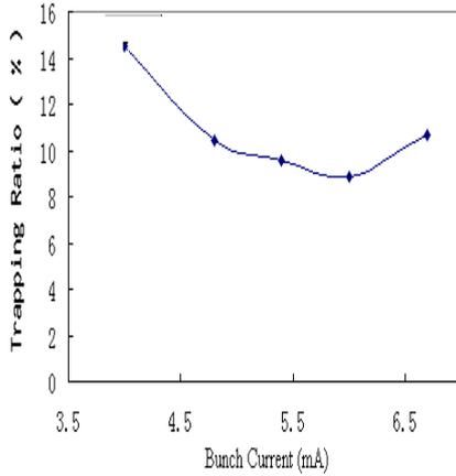
Figure 2:  $CO^+$  trapping ratio vs. bunch current
