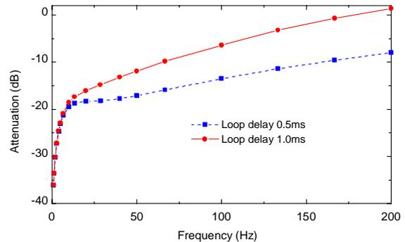
Figure 2. Noise attenuation of the closed feedback loop
