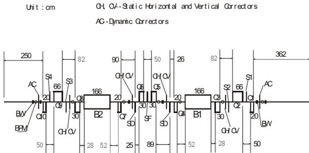
Figure 1. Layout of one DBA cell of the storage ring
