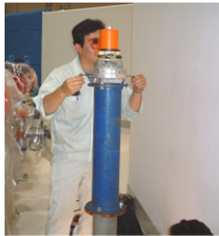
Fig.7 Centering by optical plummet on the auxiliary pillar
