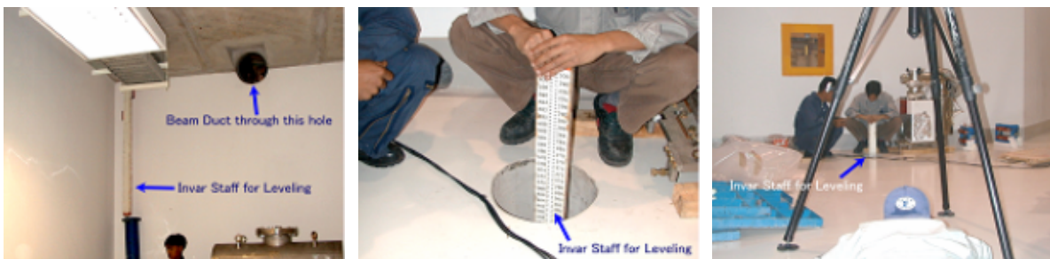
Fig.10 The Invar Staff comes through the floor hole from the downstairs in order to connect to the height between downstairs and upstairs.
