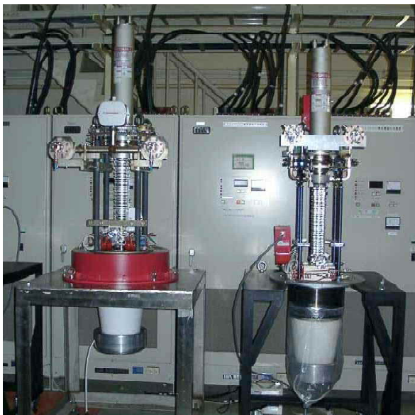
Figure 1: Photos of the PPM-1 (right) and PPM-2 (left) klystrons.
