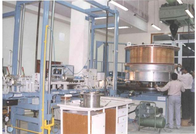
Figure 5 : Superconducting coil winding setup at VECC.
