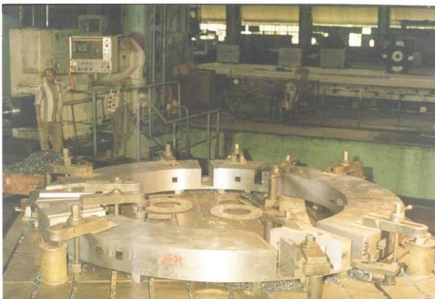
Figure 4 : Machining of the central return path ring for the main magnet frame.
