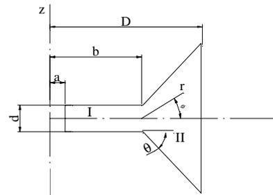
Figure2: Drawing of the coupling cavity
