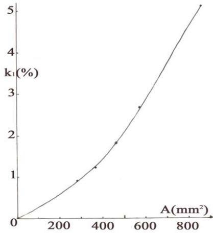
Figure3:  $k_1$  verse coupling slot area
