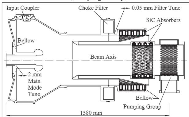
Fig. 4 Single-mode cavity for NANO HANA
