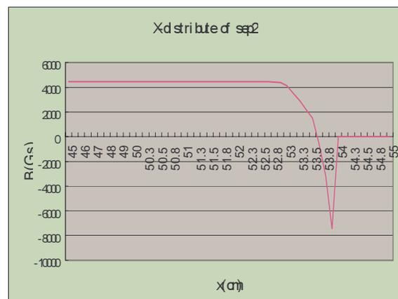
Fig3. 2-D field distribution of CSRm Ex. Septum along X-direction
