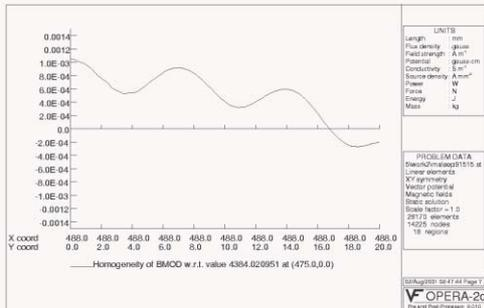
Fig6. Optimized field distribution near septum leg along Y-direction
