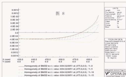
Fig7. Optimized field distribution in aperture along X-direction
