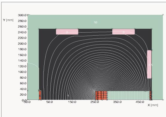
Fig2. Cross-section field distribution of CSRm Ex. septum
