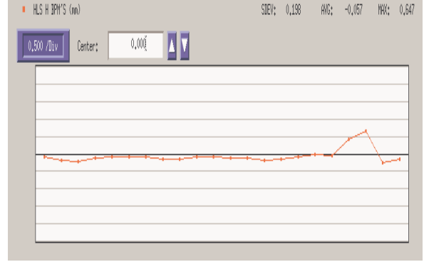
Fig 2 Local Bump in horizontal plane with Corrector CQ4N, CQ5N and CQ8N
