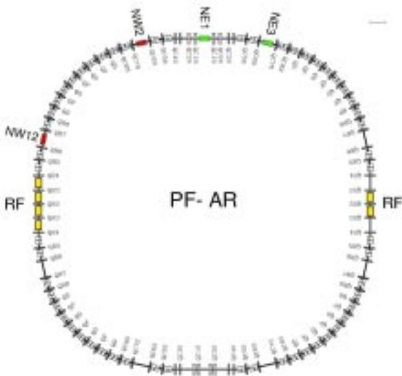
Figure 1: The lattice configuration of the PF-AR. The NE1 and NE3 indicate the existing insertion devices, and NW2 and NW12 indicate new ones.
