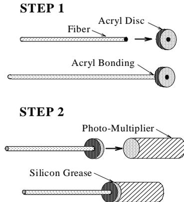
Figure 2: Method used to connect a photo-fiber to a photo-multiplier
