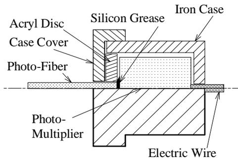
Figure 1: Cross section of a loss monitor composed of a photo-fiber, a photo-multiplier and an iron case
