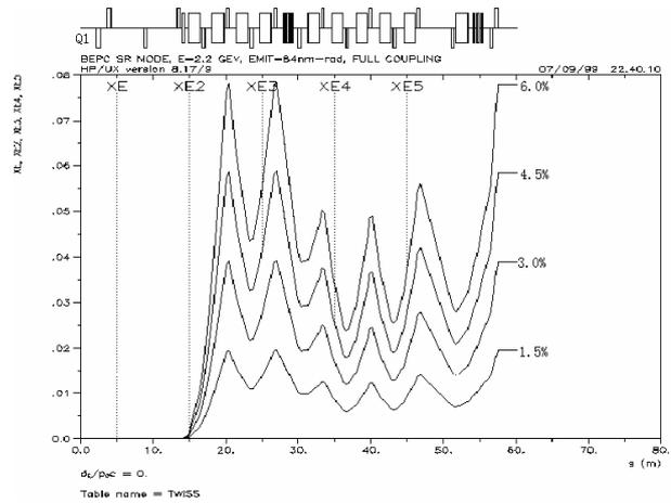
Figure 2: The path of electrons through a FODO structure with an energy loss of  $\Delta E/E = 1.5\%$  to  $6\%$ .
