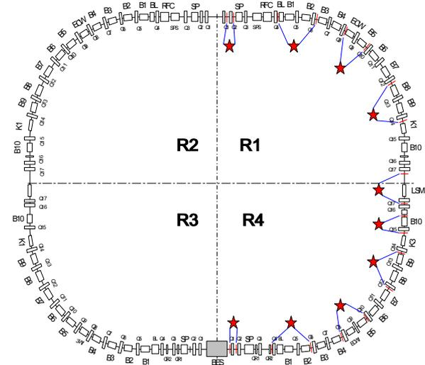
Figure 1: Distribution of Beam Loss Detectors along the BEPC storage ring
