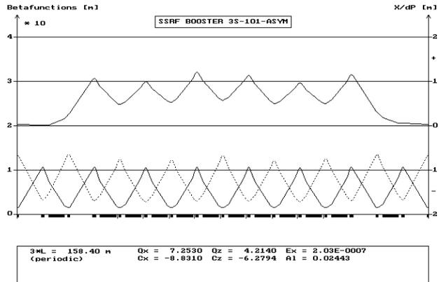
Fig.3  $\beta$  functions and dispersion function of Booster
