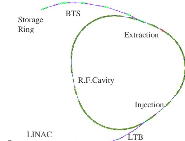
Fig.2 The Schematic layout of SSRC injector
