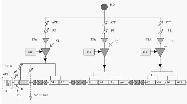
MO: Master oscillator, ATT: Attenuator, B: Buncher
