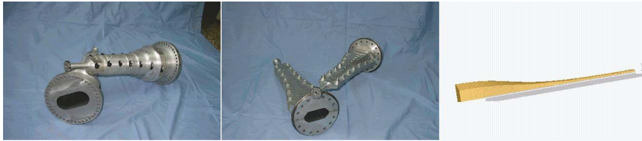
(a) taper for BEPC beam pipe shape (b) taper for SSRC beam pipe shape (c) the inner surface of the taper Figure 3: The taper matching section
