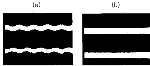
Figure 2: Beam oscillations in 2.5 GeV that are observed in streak camera. (a) the number of bunches are 468, 115 mA, \nu_x=14.26 and \nu_y=8.15 . (b) the number of bunches are 400, 110 mA \nu_x=14.28 and \nu_y=8.18 .
