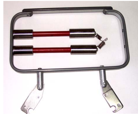
Fig.2. Glass-glaze resistor unit
