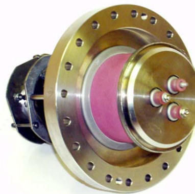
Figure 2: Picture of ion source prototype (rear view)
