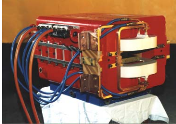
Figure 7: The booster dipole prototype.
