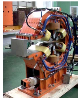
Figure 5: The storage ring sextupole prototype.
