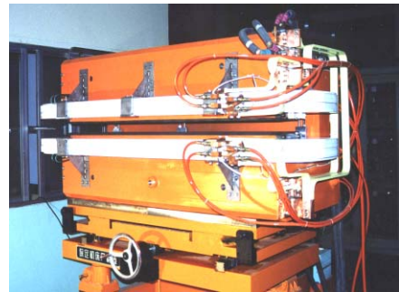
Figure 1: The storage ring dipole prototype.
