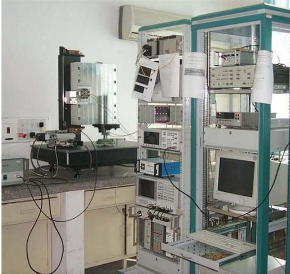
Figure 2: The calibration stand of SSRF BPM
