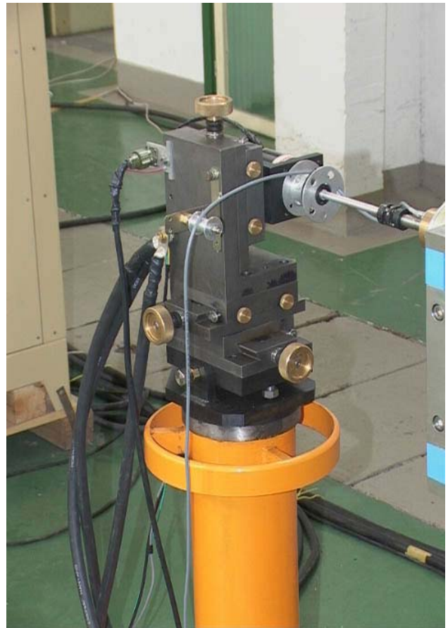
Figure 4: Motor holder of the rotating coil magnetic measurement system
