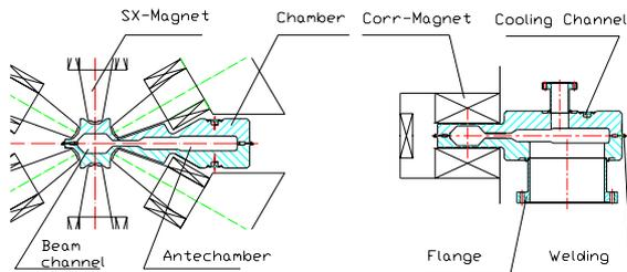
Figure 2: Cross-section of the vacuum chamber
