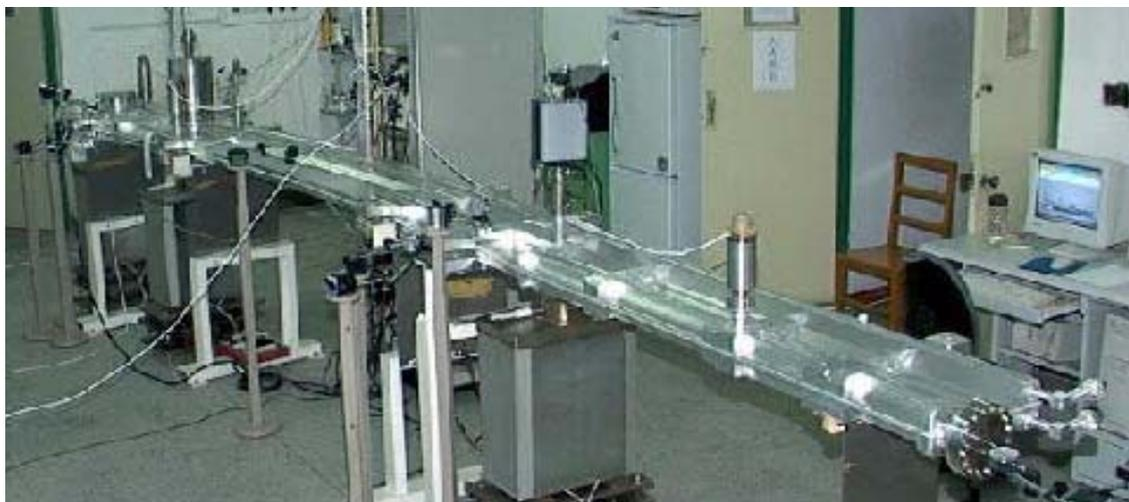
Figure 1: The prototype of UHV chamber for the SSRF storage ring
