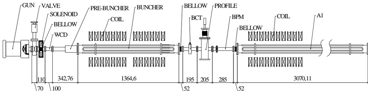
Fig.1. Pre-injector of the SSRF linac
