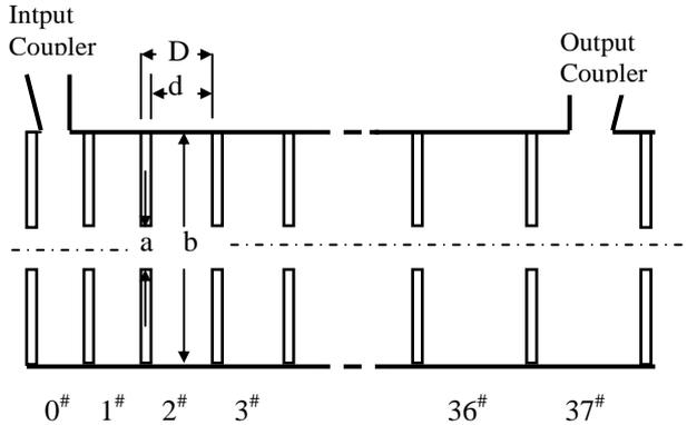
Fig. 4. Schematic structure of the buncher
