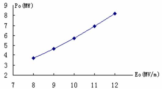
Fig.5. Input power for different accelerating field
