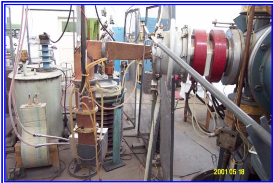
Fig 1: The ECR proton source in CIAE
