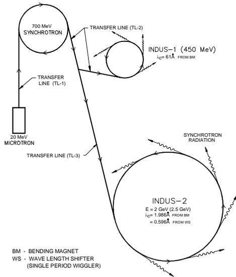
Figure 2 : Schematic Layout of Synchrotron Radiation Sources Indus-1 and Indus-2
