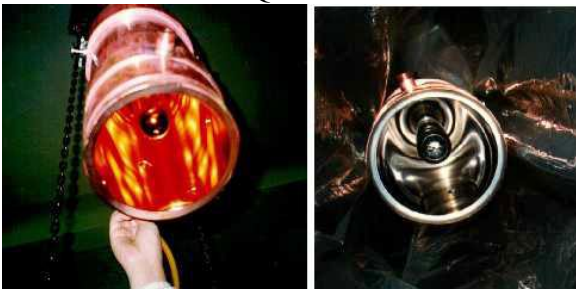
Fig. 11 QWR before (left) and after niobium sputtering
