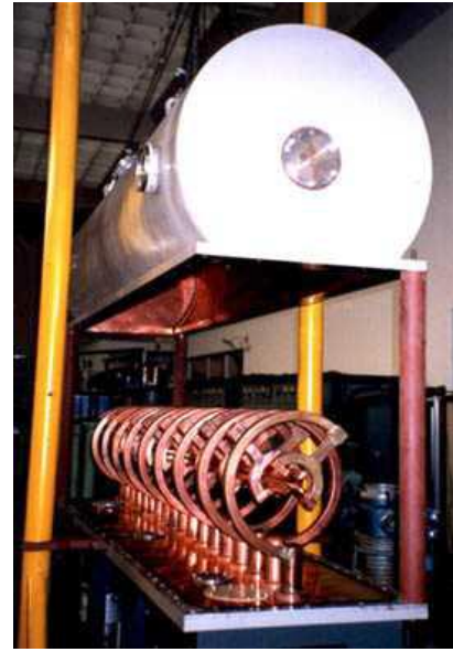
Fig. 2 Structure of ISR RFQ-1000 660 μA and a beam efficiency of 83%, while for N + and O + ions, they are 300 μA and 320 μA respectively, both with an efficiency of 86%. Detailed results are shown in Tab. 2.
