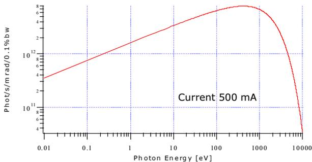
Fig. 4: Bending spectrum of Helios 2
