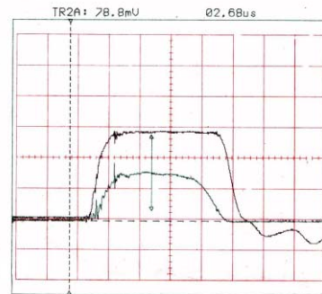
Figure 4: Upper trace is Magnetron anode voltage pulse at 41kV and Lower trace is microwave pulse at 2MW power level on a microwave load horizontal scale is 1microsecs/div.
