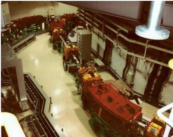
Fig. 8: A synchrotron ring and a part of a high energy beam transport line of Hyogo Ion Beam Medical Center.
