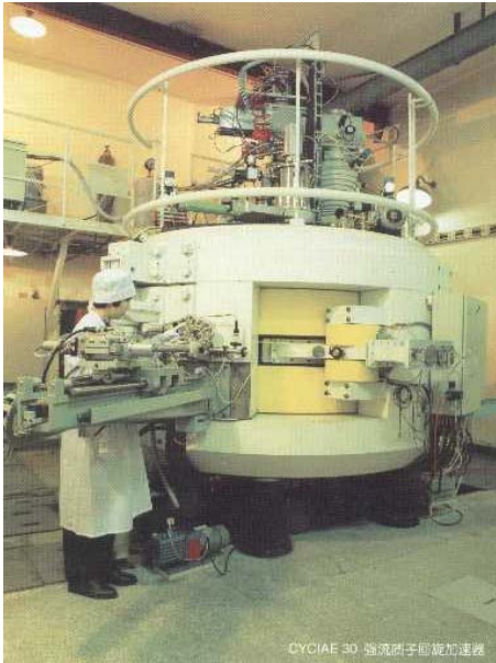
Figure 6: 30MeV Cyclotron (CYCIAE-30) made by CIAE.
