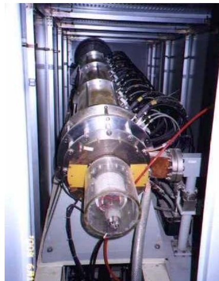
Figure 10: 9 MeV TW linac from the electron gun side.
