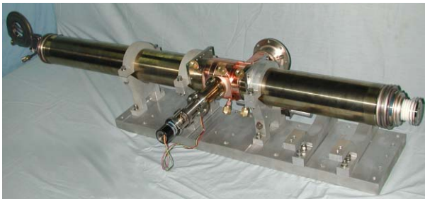
Figure 1: 20 MeV SW medical acceleration tube with an "energy switch".
