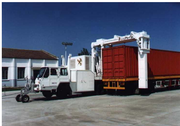
Figure 12: mobile container inspection system
