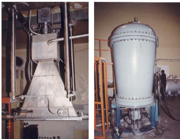
Figure 9: The 800~1200 KV 80 mA accelerator at LIMPR
