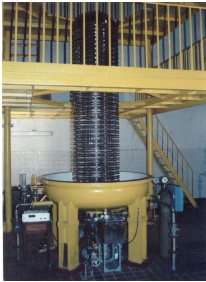
Figure 4: 3.0MeV Dynamitron-type machine made by SINR.
